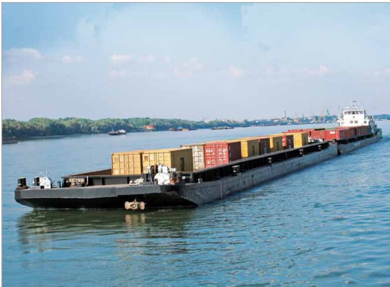
Push boat Georgi Izmirliiev type with power 1 740 hp container transport on the line Constantza - Belgrade
