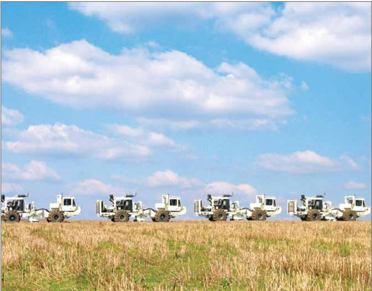
New generation seismic vibrators I/O AHV - IV 362 for 2 - D u 3 - D seismic research
