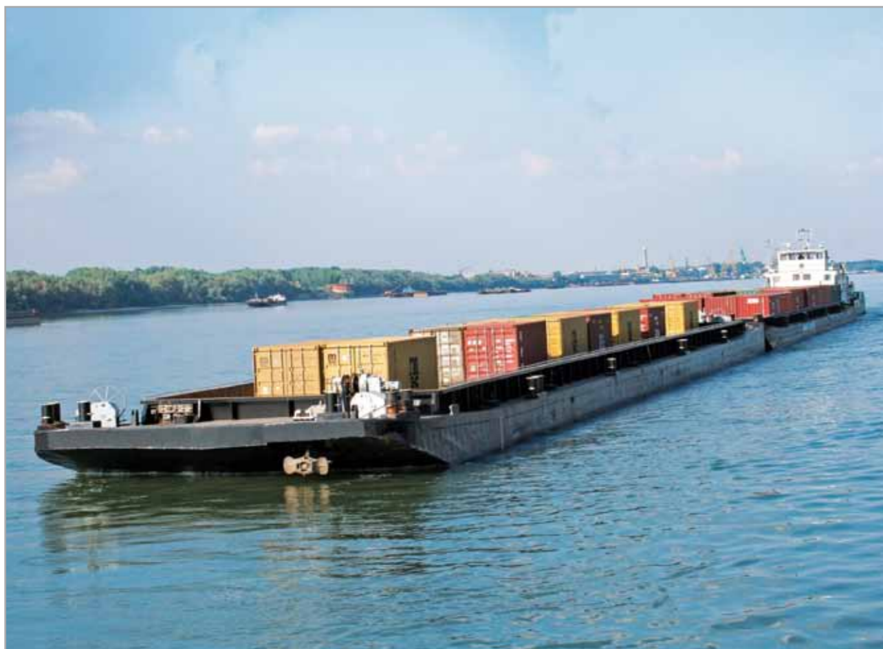
Push boat Georgi Izmiriev type with power 1 740 hp container transport on the line Constantza - Belgrade
