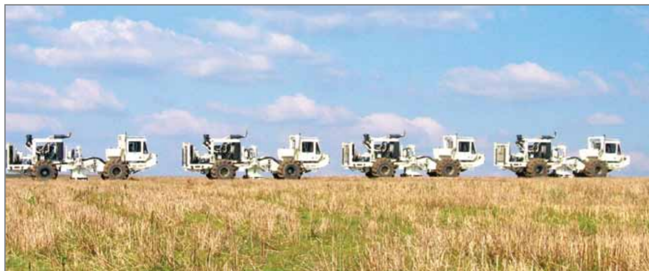
New generation seismic vibrators I/O AHV - IV 362 for 2 - D u 3 - D seismic research
