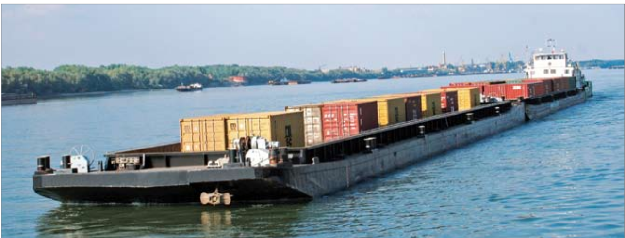
Push boat Georgi Izmirliiev type with power 1 740 hp container transport on the line Constantza - Belgrade
