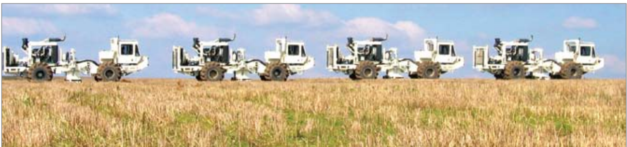
New generation seismic vibrators I/O AHV - IV 362 for 2 - D u 3 - D seismic research
