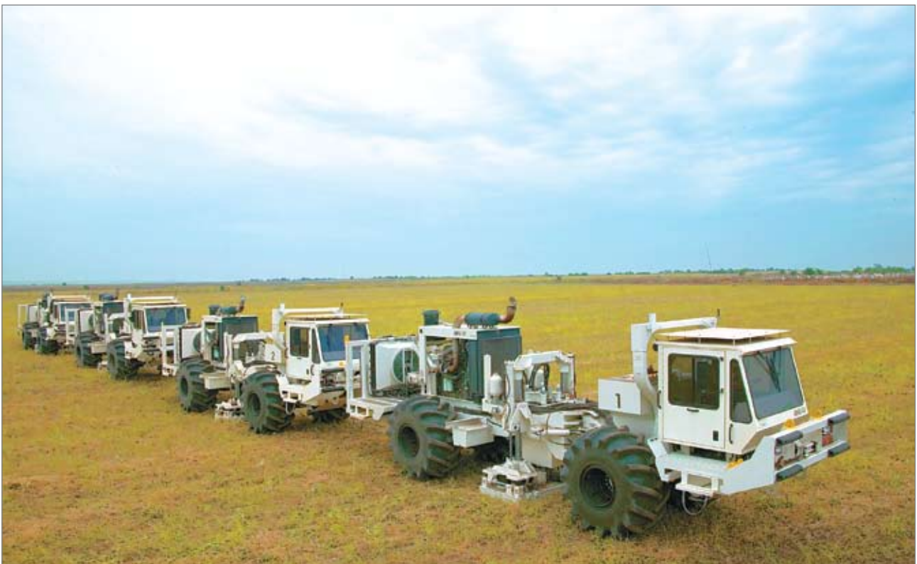
New generation seismic vibrators I/O AHV - IV 362 for 2-D u 3-D seismic research
