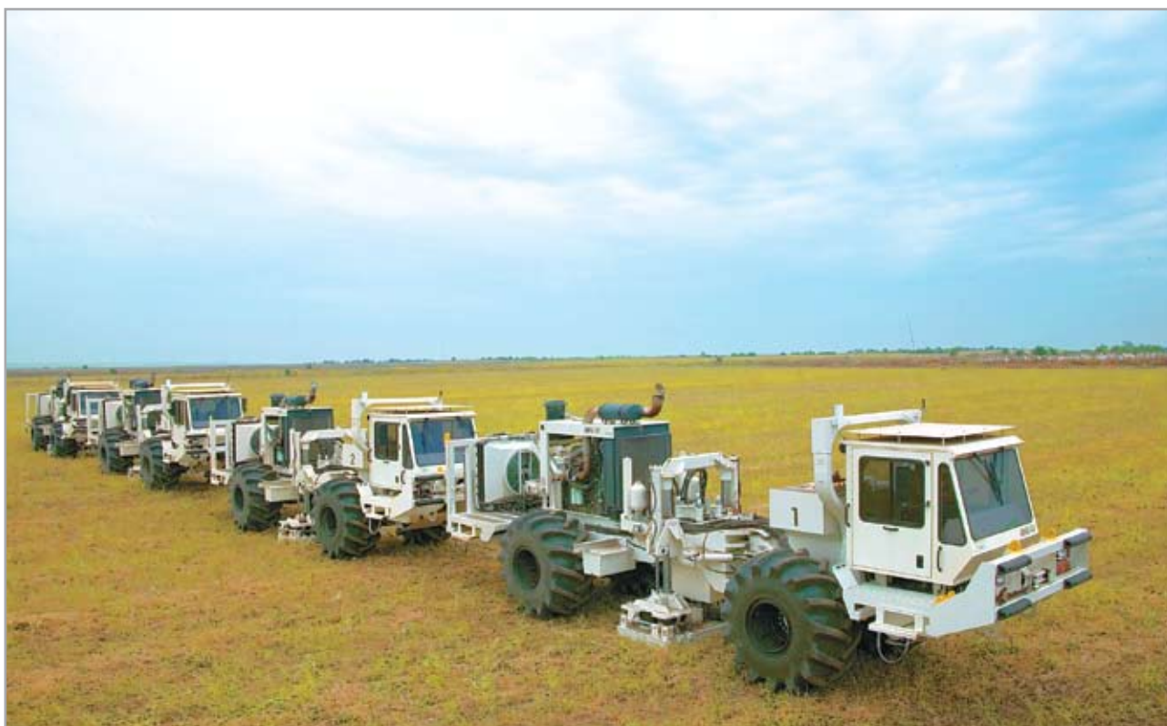
New generation seismic vibrators I/O AHV - IV 362 for 2-D u 3 - D seismic research
