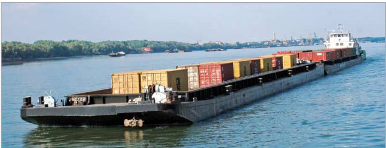
Push boat “Georgi Izmirliev” type with power 1 740 hp container transport on the line Constantza - Belgrade
