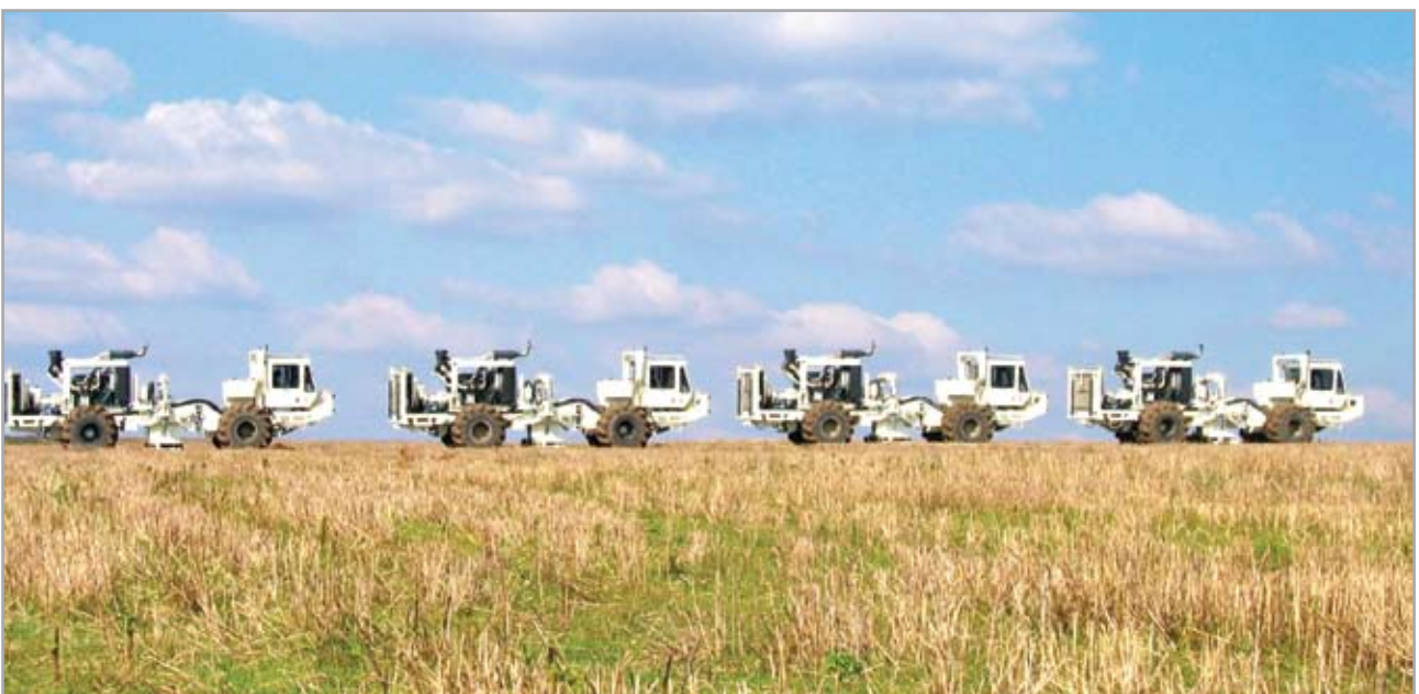
New generation seismic vibrators I/O AHV - IV 362 for 2-D u 3 - D seismic research
